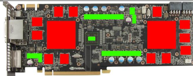
Apply a thin layer of thermal compound to the GPUs and the RAM modules. These components are marked red in the figure. The thermal compound must not be electrically conductive! Cut fitting pieces from the thermally conductive pad supplied with the aquagraFX and place them on top of the components indicated by green rectangles.
