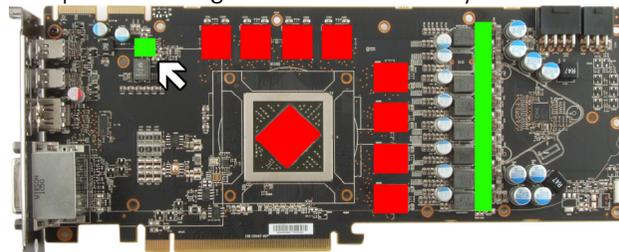
Apply a thin layer of thermal compound to the GPU and the RAM modules (indicated by red marks in the figure). The thermal compound must not be electrically conductive! Cut fitting pieces from the thermal pad supplied with the waterblock and place them on top of the voltage regulators (indicated by green marks in the figure).
