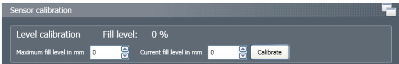
Before the sensor can produce accurate readings, it needs to be calibrated. To do so, use a folding rule or measuring tape to determine current fill level and maximum fill level of your reservoir and enter the values into the corresponding boxes of the software. After confirming these values by clicking "Calibrate", the software will generate the calibration data.
